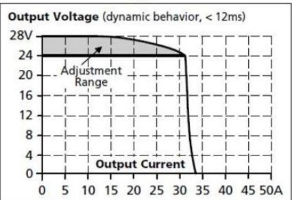
Fig. 6-1 Output voltage vs. output current, typ.
