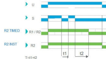
Function Ht - Interval summation time relay
