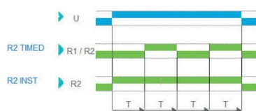
Function D - Symmetrical flashing (OFF Start)
