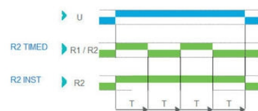
Function Di - Symmetrical flashing (ON Start)
