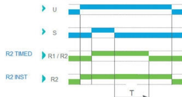
Function C - Off-Delay (Delay on break)
