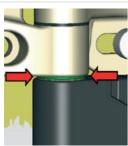
4. The bolt is tightened until the red indication disk between the hinge and switch unit is replaced with a green indication disk. Secure with extra 2 Nm (+10 %). Safety hinge is now operational and the contacts open while the door is opened.
