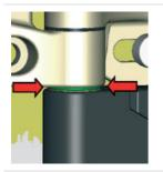
4. The bolt is tightened until the red indication disk between the hinge and switch unit is replaced with a green indication disk. Secure with extra 2 Nm (+10 %). Safety hinge is now operational and the contacts open while the door is opened.
