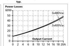
Fig. 11-2 Losses vs. output current at 48V,
