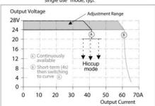
Fig. 6-4 Dynamic overcurrent capability, typ.
