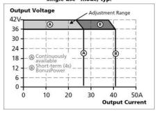
Fig. 6-4 Dynamic overcurrent capability, typ.
